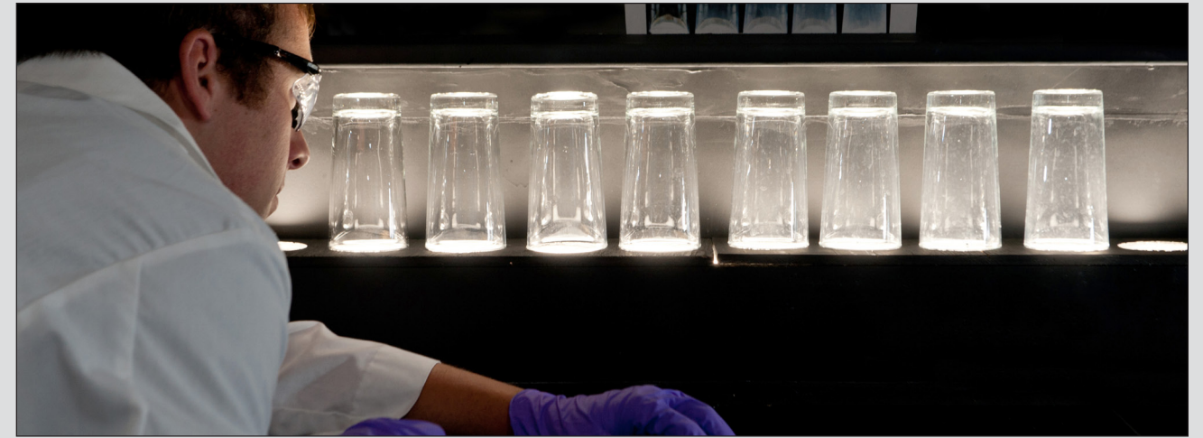
Rivertop Research Chemist Erik Johnston measures the spotting and filming on drinking glasses cleaned in a dishwasher with Rivertop’s “green” phosphate replacement.
